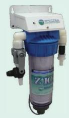
The Z-lon uses bimetallic ions to disinfect your entire watermaker, including the filters and membranes. It prevents bacteria growth for up to a month and eliminates the "pickling process." The Z-lon is completely automatic and energy efficient, drawing only 15 watts during the fresh water flush cycle and less than one watt in stand-by. All Spectra Watermakers are retrofittable for the Z-lon.
