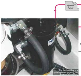
The only slight issue with our system is that, due to its location low down in the engine room, it is quite hard to drain and we have had to attach a hose to the valve as there isn't enough room to slide a bowl underneath.
